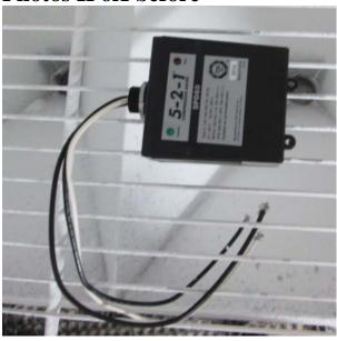
IP6X After – Unit is hermetically sealed therefore no dust could enter the enclosure.
