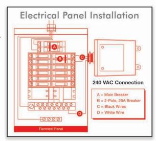
All conductor lengths should be as short as possible and bends should not be sharp; a 4" bend radius or wider is recommended.
